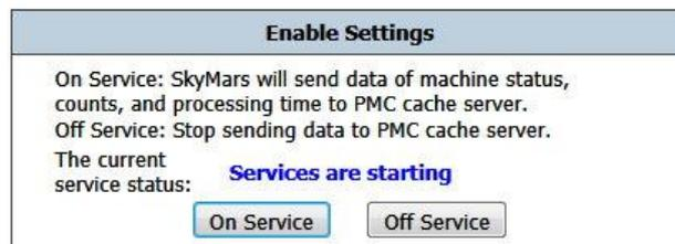
[On Service] : Open utilization rate view, and then SkyMars will transmit data (the machine status) to a flash server of PMC (PMC cache server) to save it temporarily. It also provides a website to read utilization rate and show on the webpage.
